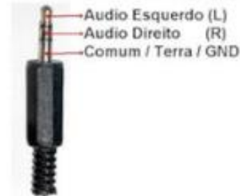
P2 - 3 pin 3.5mm (2.5mm) plug connector
