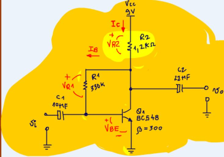
$$I_B = \frac{V_{CC} - V_{BE}}{\beta R_2 + R_1}$$
