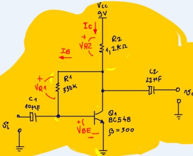
$$I_B = \frac{V_{CC} - V_{BE}}{\beta R_2 + R_1}$$
