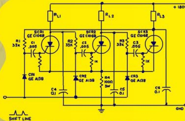
FIGURE 8.22 CATHODE COUPLED RING COUNTER
