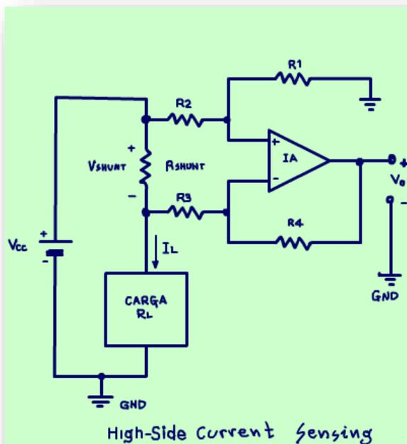
$$V_{CM} = V_{CC} \frac{R_1}{R_1 + R_2}$$
